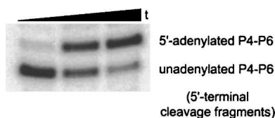
FIGURE 4. 5'-Adenylation of P4-P6, a long and structured RNA substrate. The 160-nt RNA substrate was 5'- 32 P-radiolabeled. Following 5'-adenylation ( t = 0 h, 8 h, and 24 h using the optimal incubation conditions of Fig. 3), the 5'-terminal 14-nt portion of the RNA was cleaved using an 8-17 deoxyribozyme (see Materials and Methods), thereby allowing the 5'-adenylation to be detected by 20% PAGE. In all lanes, the band corresponding to the 146-nt 3'-portion of the P4-P6 RNA is present near the wells (not shown).
